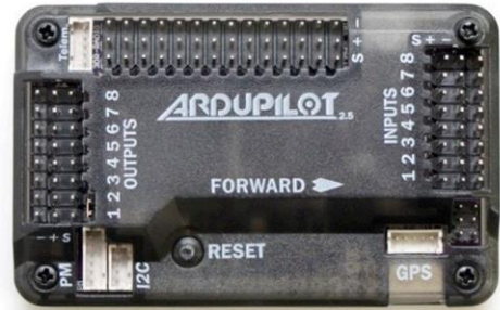
Fig.8: Ardupilot Mega 2.5 connection ports
