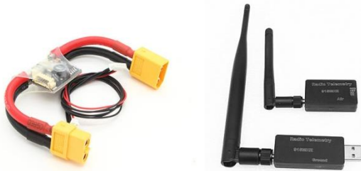
Fig.6: 3DR Power Module (left), 915 MHz Telemetry (right)
